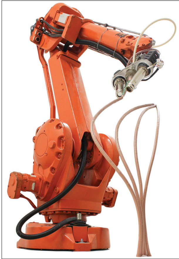
Figure 1.3 Mataerial multi-axis 3-D printer (source: Mataerial home page, accessed April 25, 2017, www.mataerial.com ).
