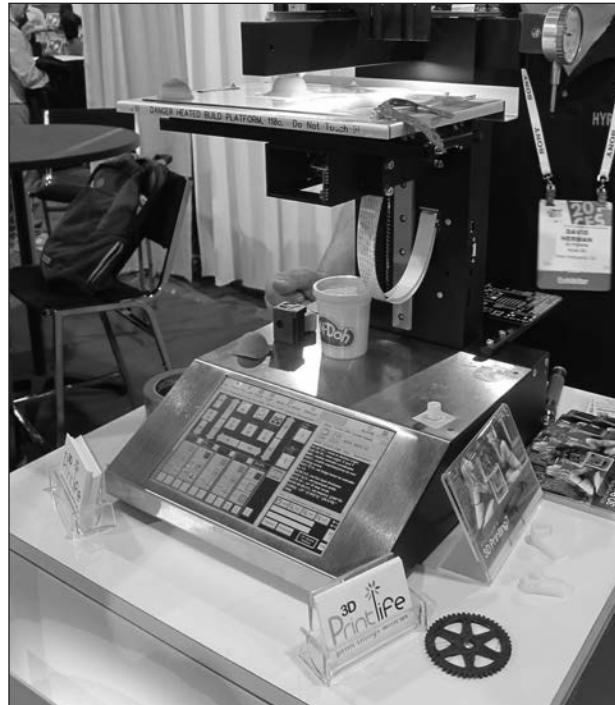
Figure 5.9 The Hyrel System 30 printing in Play-Doh
