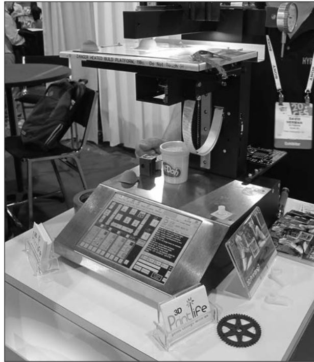
Figure 5.9 The Hyrel System 30 printing in Play-Doh
